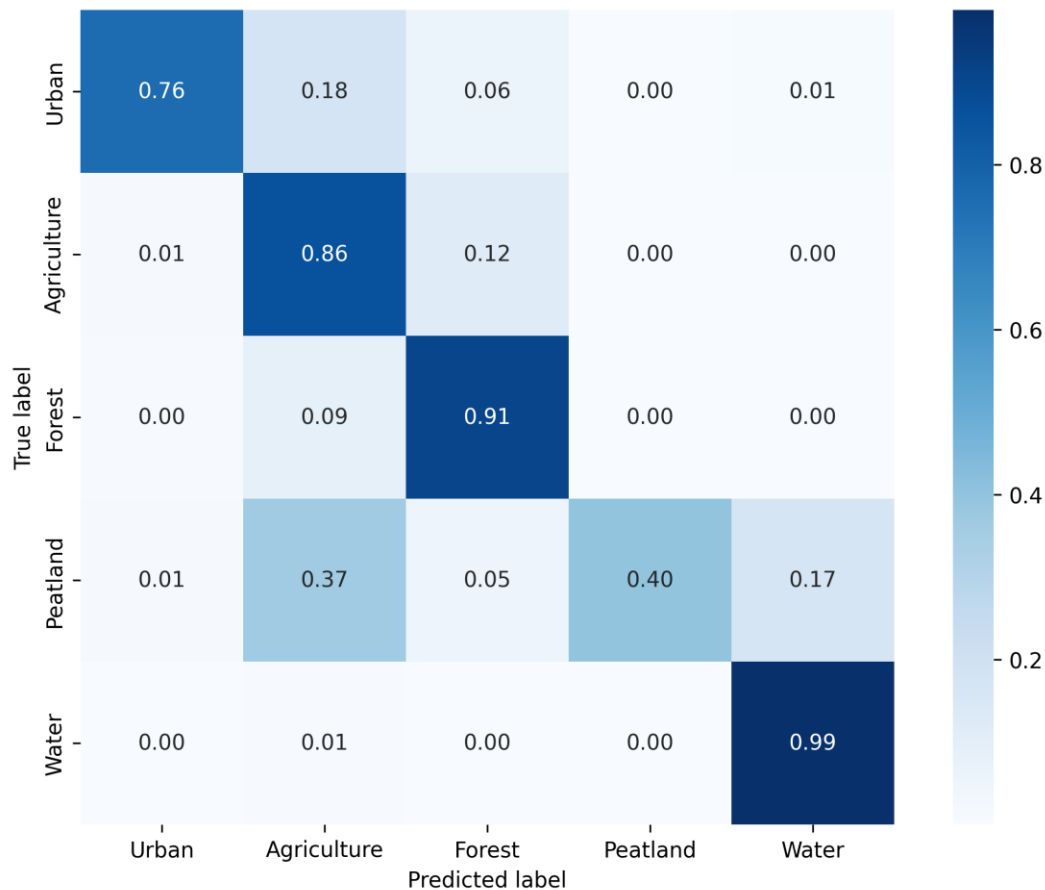
Figure 5: Confusion matrix obtained by the proposed PPLiteSeg-ASFEM model on the TurkeySAR dataset.
